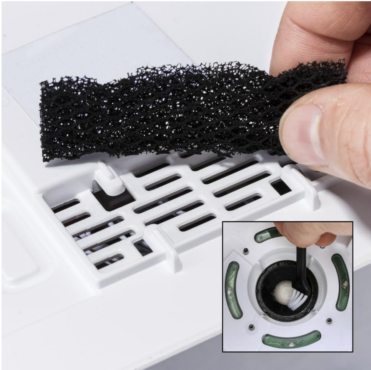
Removing the pre-filter and using the cleaning brush for the nebulizer.
