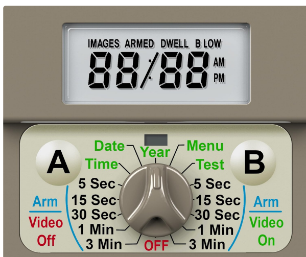
Figure 4.4: Close-up of the control dial and LCD screen, displaying settings like Date, Time, Year, Menu, Test, and
