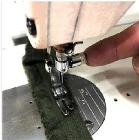
Image 2: A detailed view of the Cutex P60555 Easy & Quick Change Spring Foot Clamp, highlighting its metal construction and quick-release lever.
