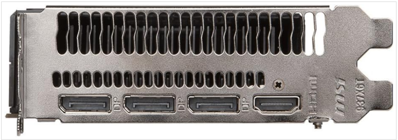
Figure 3: Display output ports (DisplayPort and HDMI) on the graphics card.
