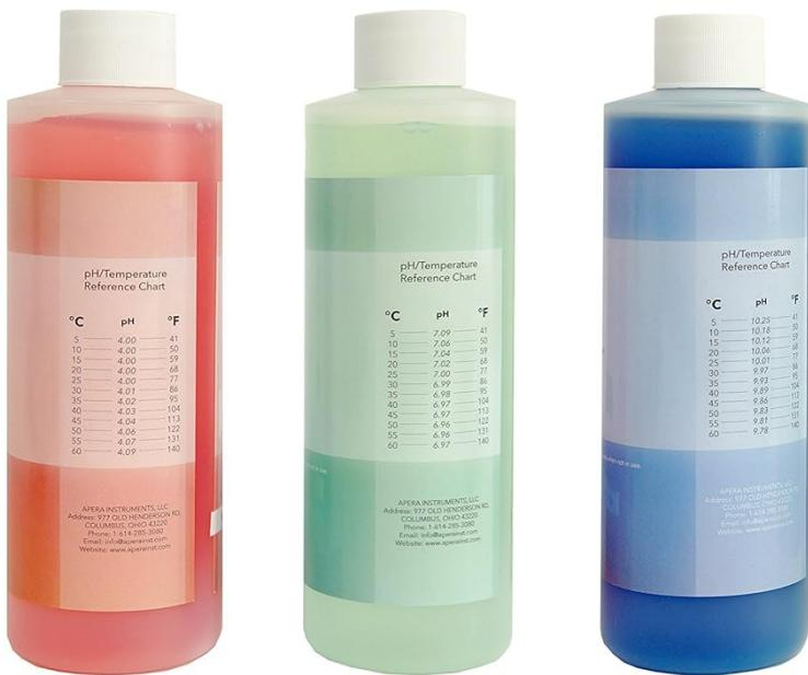
A close-up view of the three primary pH calibration buffer solutions provided with the kit, color-coded for easy identification and labeled with their respective pH values.
