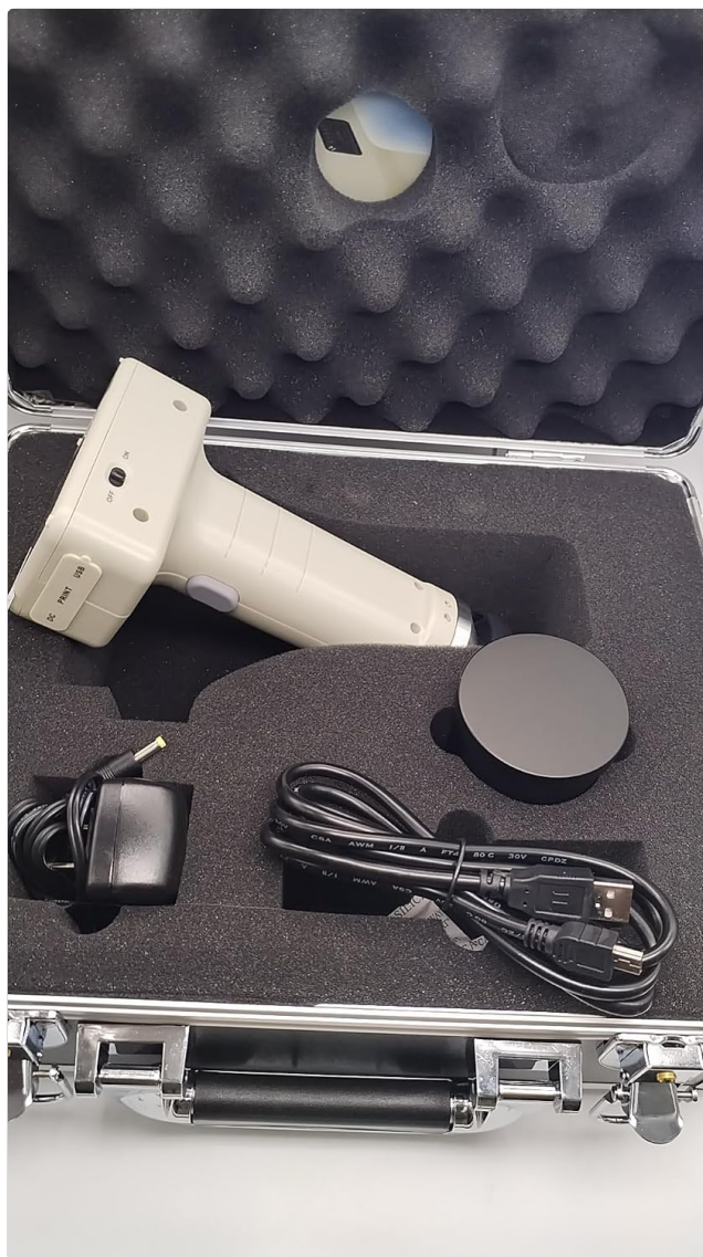
Figure 6.1: JZ-350 Colorimeter with the protection cap removed, revealing the measuring aperture.
