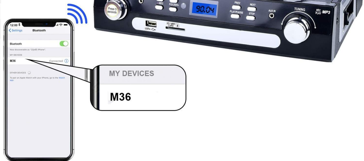
Figure 6.2: The record player in Bluetooth mode, demonstrating how to pair with a mobile device. The phone screen shows 'M36' as a discoverable device.
