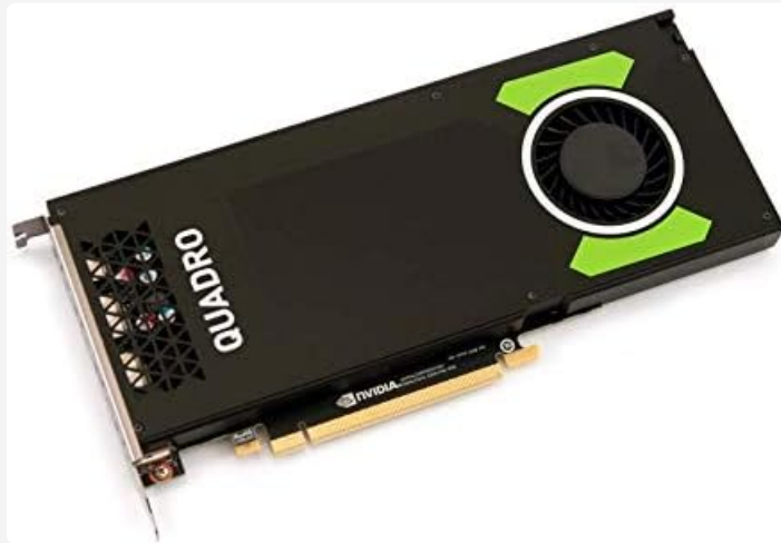
Figure 3.1: Angled view of the PNY NVIDIA Quadro P4000 graphics card, showcasing its single-slot design and cooling fan.
