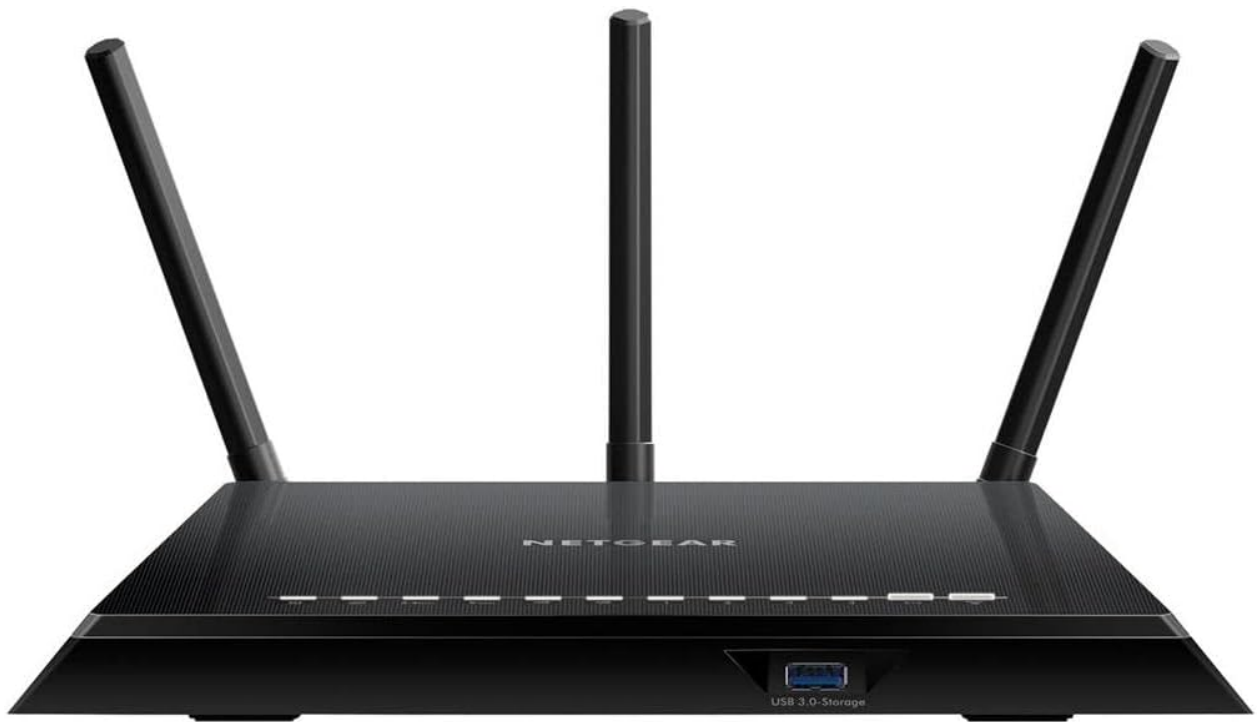
Front View: Displays the NETGEAR logo, status indicator lights for power, internet, Wi-Fi bands (2.4GHz and 5GHz), USB, and Ethernet ports, along with a USB 3.0 storage port.
