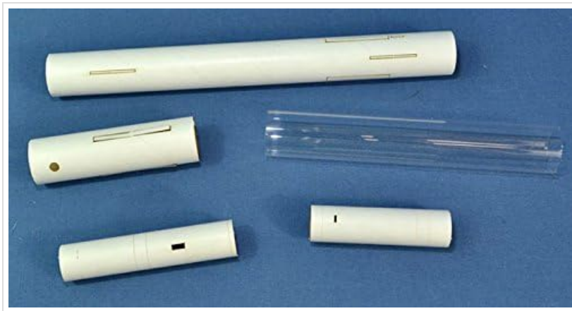
Figure 4: Different body tube components and the clear payload section, ready for assembly.
