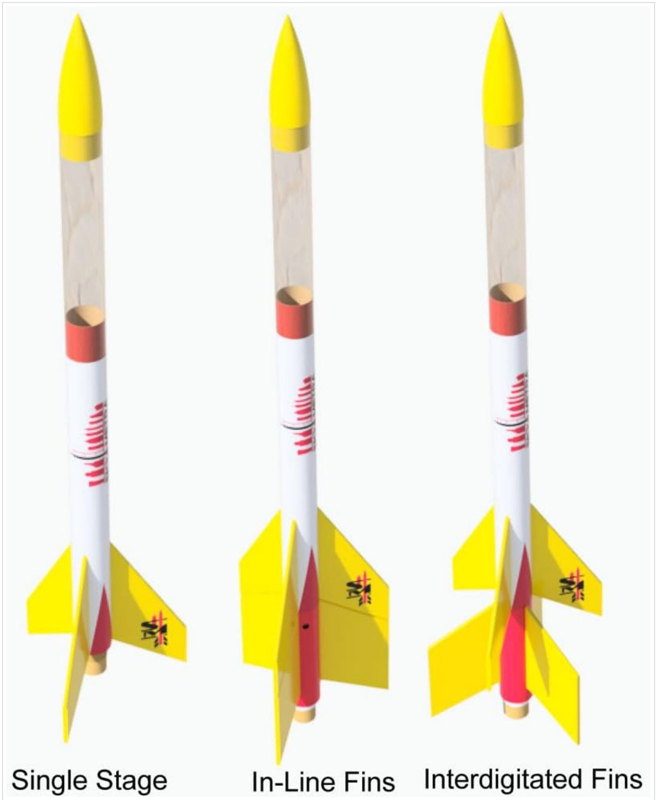
Figure 7: Illustration of different fin configurations, including the in-line fin setup used for the SkyMetra's two-stage design, which enhances stability.
