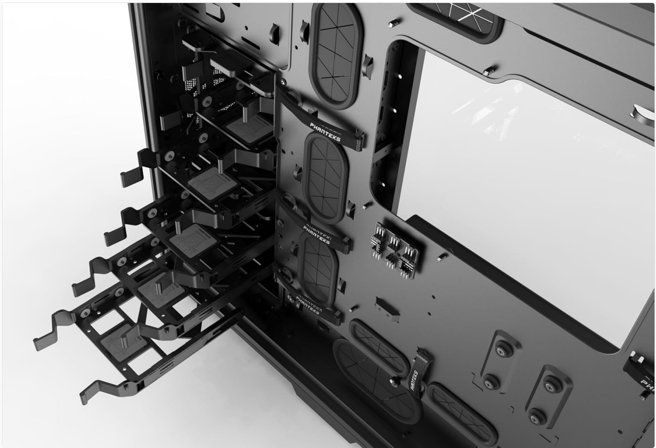
Figure 4.2: Rear of the motherboard tray, showcasing the cable management channels and Velcro ties for a tidy build.
