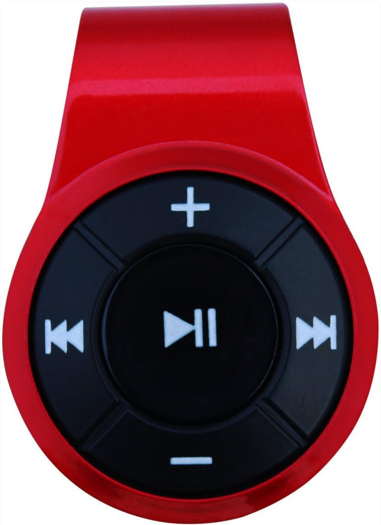
Image 2.2.1: Front view of the Bluebyte Bluetooth Receiver, highlighting the central Play/Pause button, surrounded by Volume Up (+), Volume Down (-), Previous Track (⏮), and Next Track (⏭) buttons. The device is red with black buttons.
