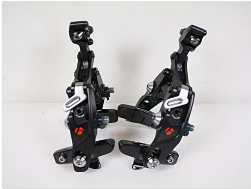
Image 4.1: Direct mount brake calipers ready for cable installation.
