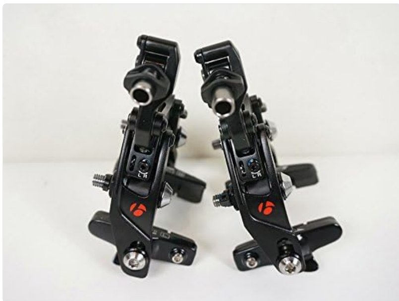
Image 4.2: Close-up of a brake caliper, showing the brake pad and its adjustment bolt.
