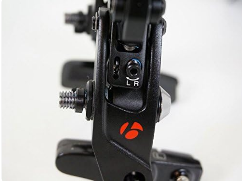
Image 4.3: Detail of the caliper, showing the centering adjustment screw (often marked L/R).
