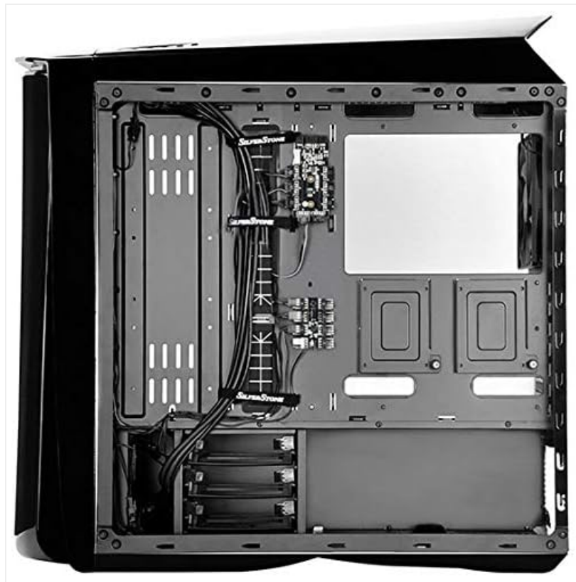
Figure 3: Internal view showing the drive bays for storage devices.
