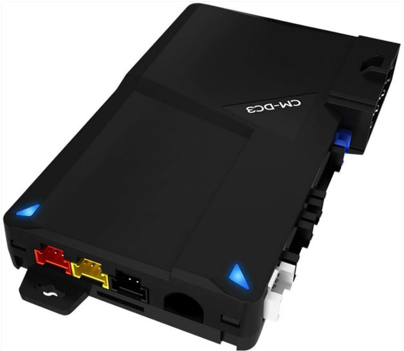
Figure 2: Close-up view of the Firstech CM-DC3 module, showing various ports and indicators.
