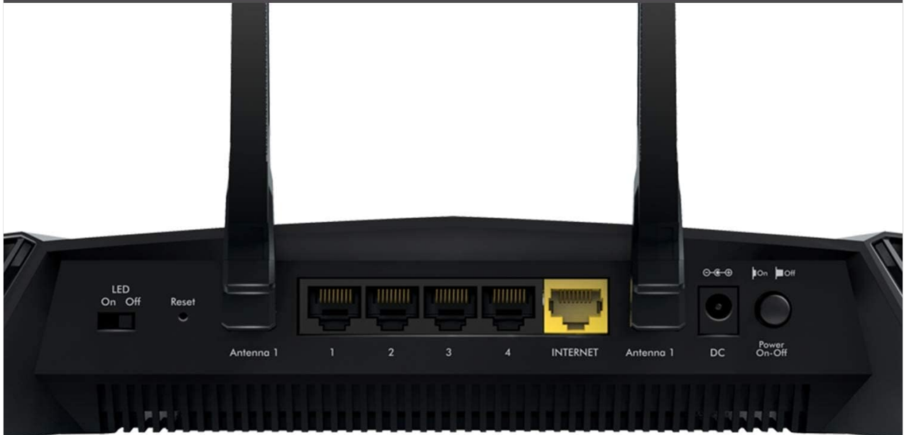
Figure 3: The rear panel of the XR500 router, illustrating the various ports for connectivity, including the WAN (Internet) port, Gigabit Ethernet LAN ports, and USB 3.0 ports.
