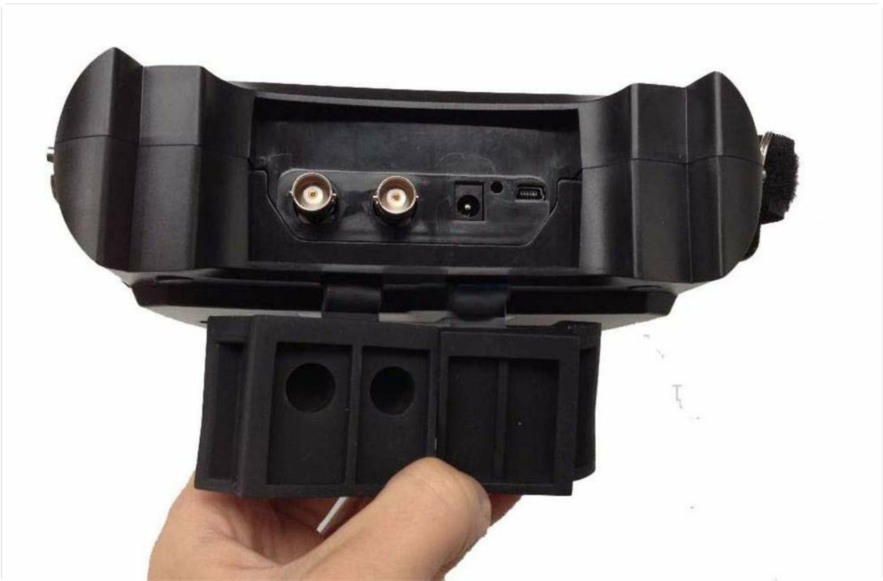
Figure 4.3: Top view of the SUB100, displaying the BNC probe connectors and USB port.
