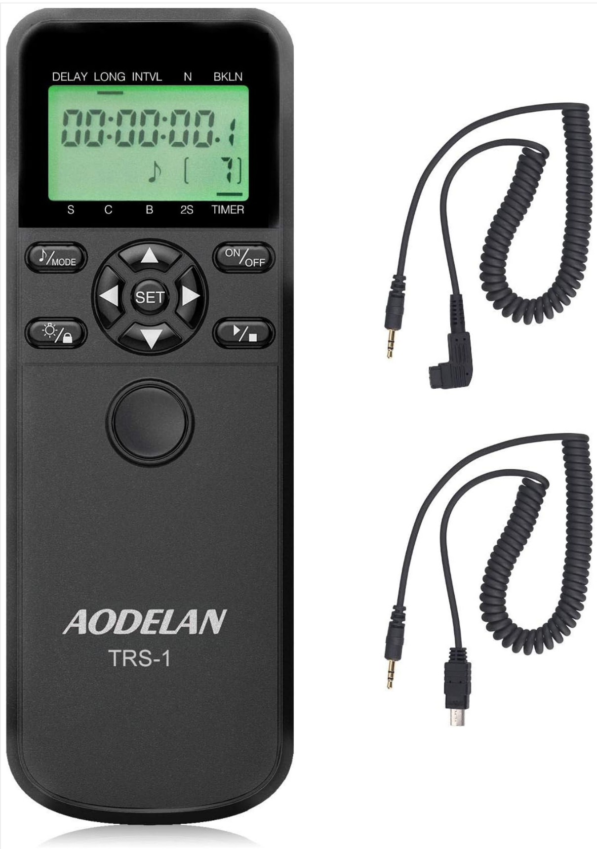
Image: The AODELAN TRS-1 remote control unit shown alongside its two coiled connecting cables, one with a right-angle connector and the other with a straight connector, both ending in a 2.5mm jack for the remote and a camera-specific connector.
