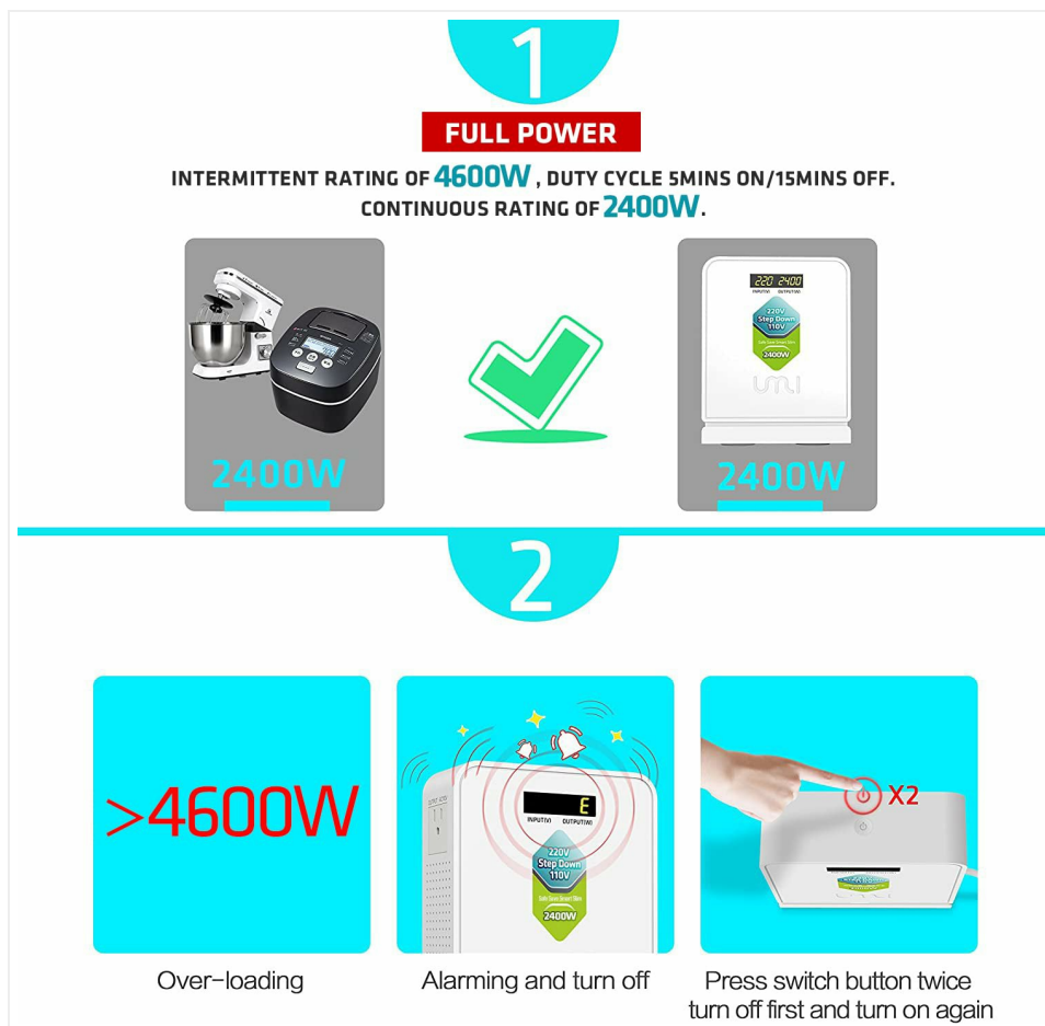
Image: Graphic explaining the continuous (2400W) and intermittent (4600W) power ratings, showing compatible appliances like a stand mixer and rice cooker.
