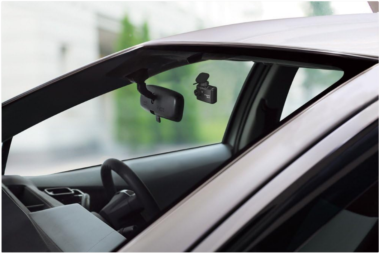
Figure 2: The Yupiteru DRY-ST1000P Drive Recorder installed on a car windshield, positioned behind the rearview mirror.
