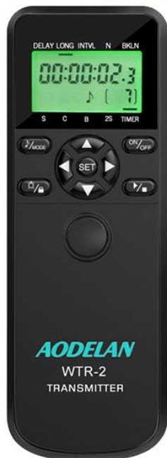
Image: The AODELAN WTR2 remote and receiver, emphasizing features such as professional anti-shake, 2.4G wireless connectivity, and a control range of 196 feet. The image also lists Bulb, Continuous, Bkln, and Timer functions.
