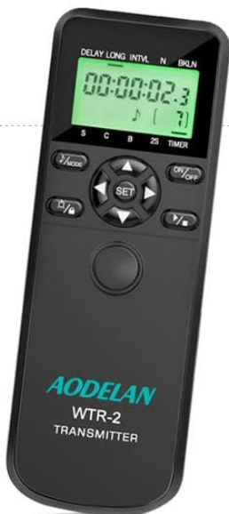
Image 5.4: Example settings for continuous shooting (Delay: 5s, Long: 0s, Interval: 2s, N: 5).
