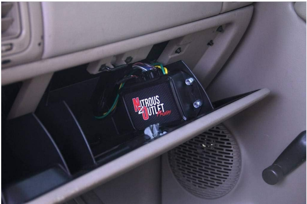
Figure 2: Example installation of the ProMax controller in a vehicle's glove compartment.
