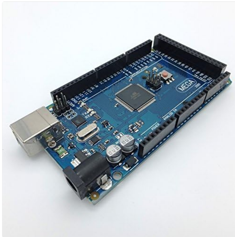
Image: The JDH Labs Tech Mega 2560 R3 compatible development board.
