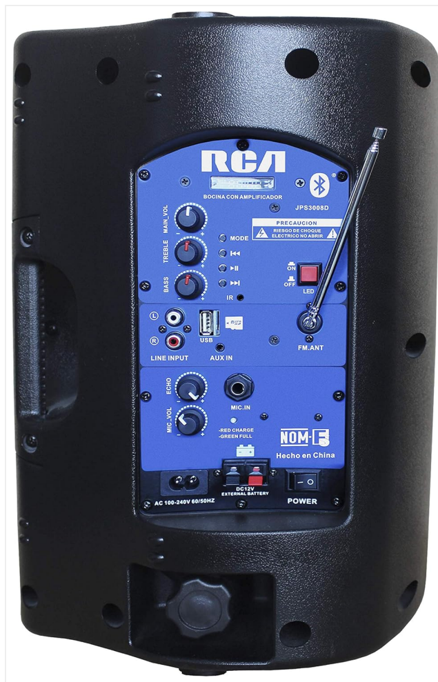
Image 2: Rear Control Panel - This image shows the detailed rear panel of the speaker. It includes knobs for Bass, Treble, Main Volume, Mic Volume, and Echo. Ports for USB, AUX In, Line Input, and Mic In are visible. There are also buttons for Mode, Play/Pause, Skip tracks, and an On/Off switch for LED lights. An FM antenna and a power input for AC 100-240V and DC 12V external battery are also present.
