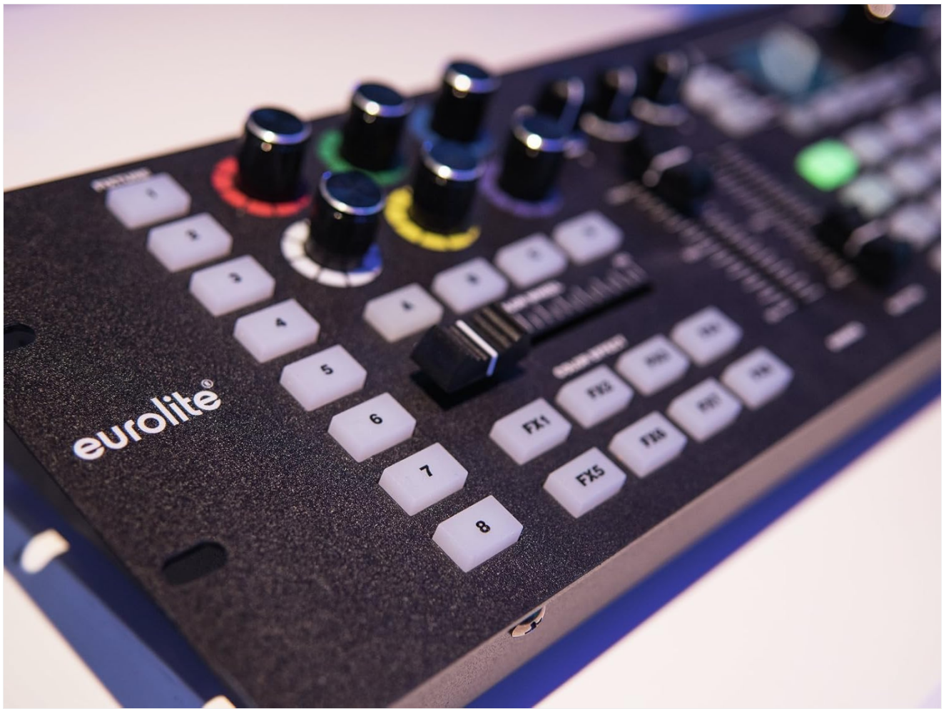
Figure 4.4: Fixture and Color Controls. A close-up view of the fixture selection buttons (1-8) and the color control section, including the color wheel fader and individual color adjustment knobs.
