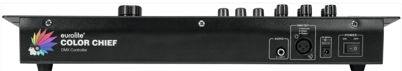
Figure 4.7: Rear Panel Connections. This image shows the rear panel of the controller, featuring the DMX OUT (3-pin XLR), Audio input (XLR), DC 9-12V power input, and the POWER ON/OFF switch.
