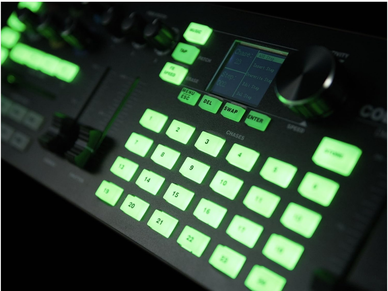
Figure 4.5: Display and Navigation. This image focuses on the central LCD display and the surrounding navigation buttons (MENU/ESC, DEL, SWAP, ENTER), which are used for menu interaction and parameter adjustments.
