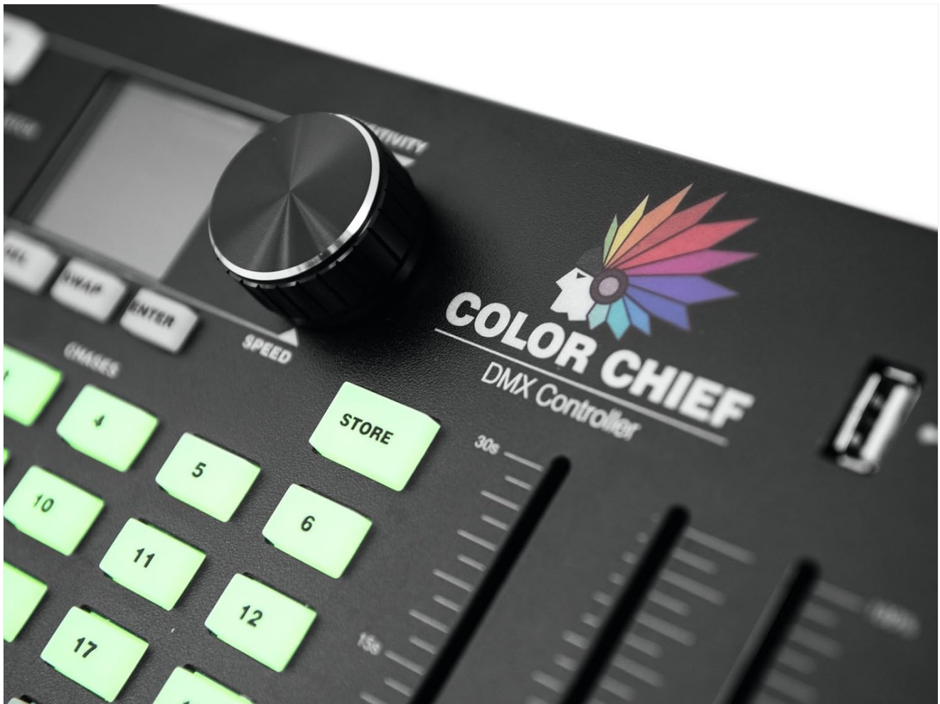
Figure 4.6: Speed and Store Controls. A detailed view of the Speed knob, used for adjusting chase or effect speeds, and the Store button, essential for saving scenes and chases.
