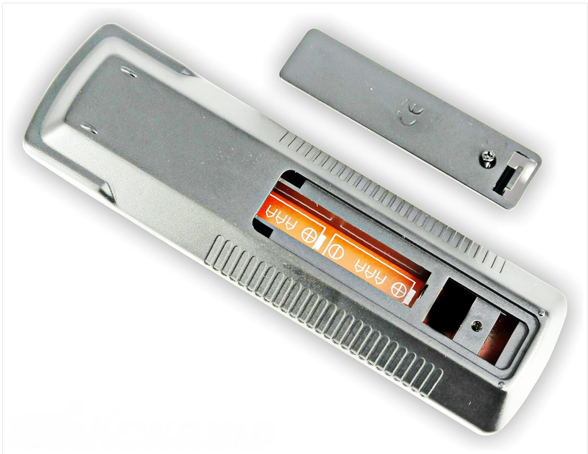
Image 2.2: The battery compartment with two AAA batteries inserted, showing correct polarity alignment.
