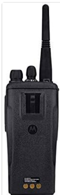
Image 5.1: Back view of the Motorola CP200d radio, showing the battery contacts and attachment points.
