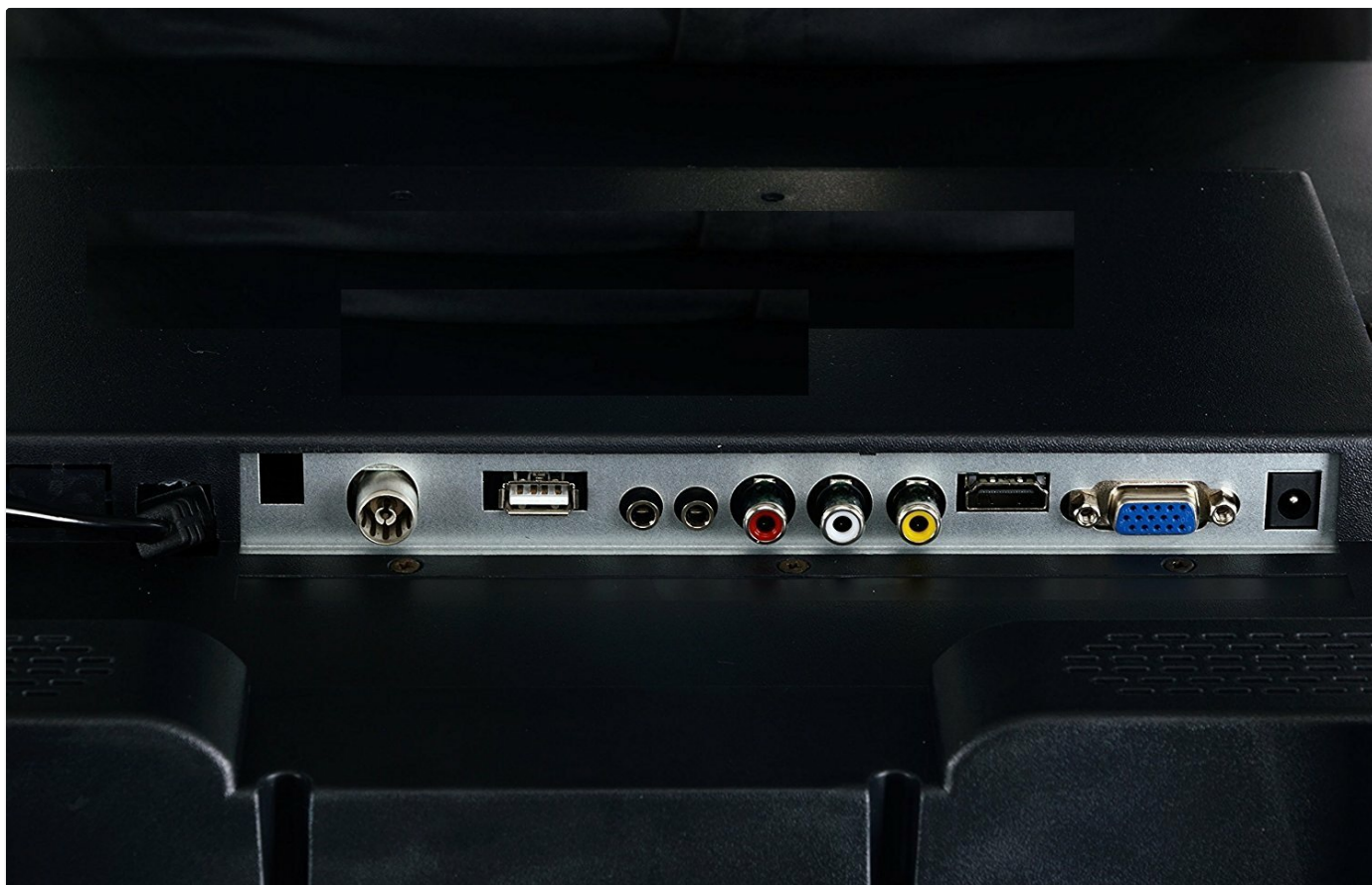
Figure 5: Detailed view of the rear input ports on the BUSH 15-inch HD LED Monitor Television, showing HDMI, USB, VGA, AV, and RF connections.
