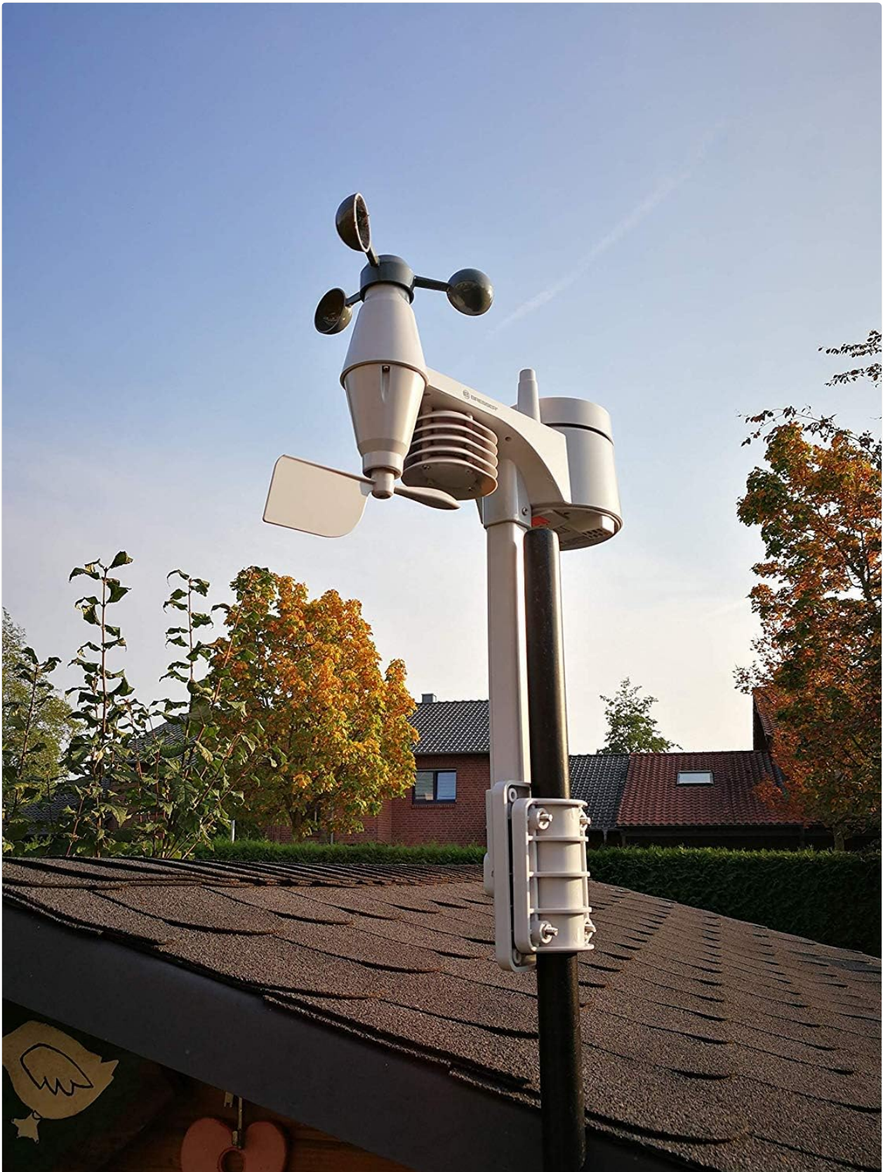
Figure 3.2: The 5-in-1 outdoor sensor correctly installed on a pole, ensuring optimal exposure for accurate weather data collection.
