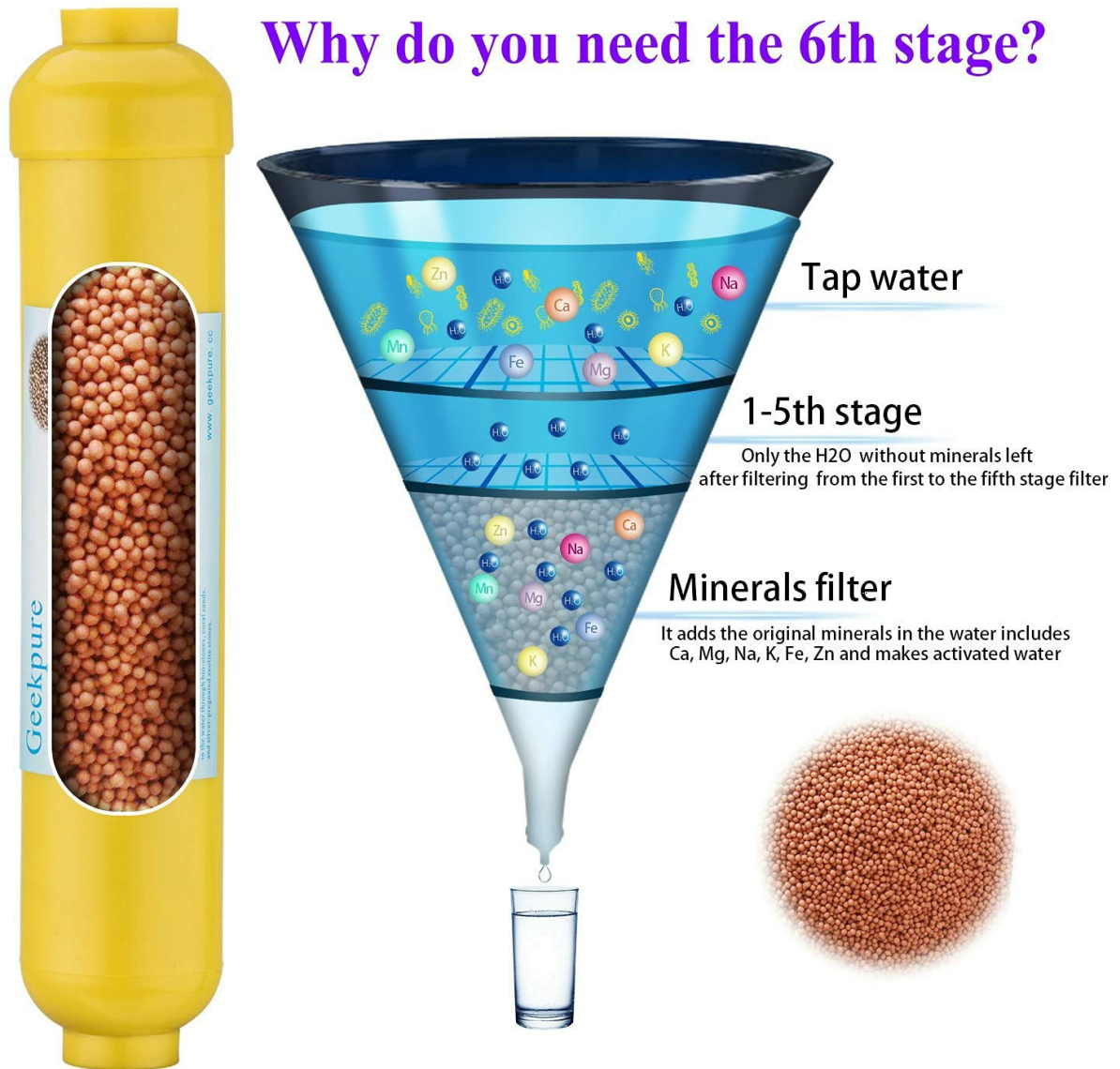
Image: Illustration demonstrating how the mineral filter reintroduces essential minerals like Calcium, Magnesium, and Zinc into the purified water.
