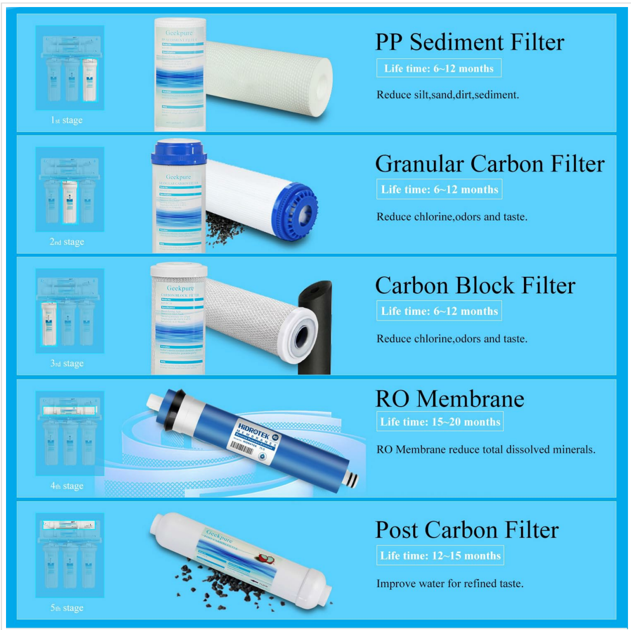
Figure 4: Five stages of filtration and filter lifetimes.
