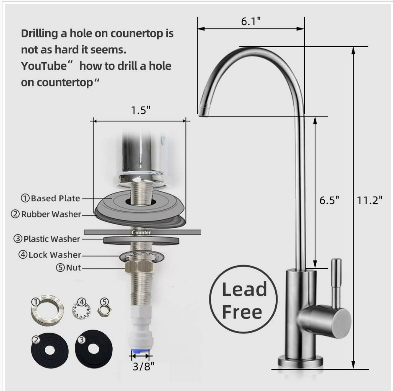
Figure 2: Faucet installation diagram, showing components and dimensions.
