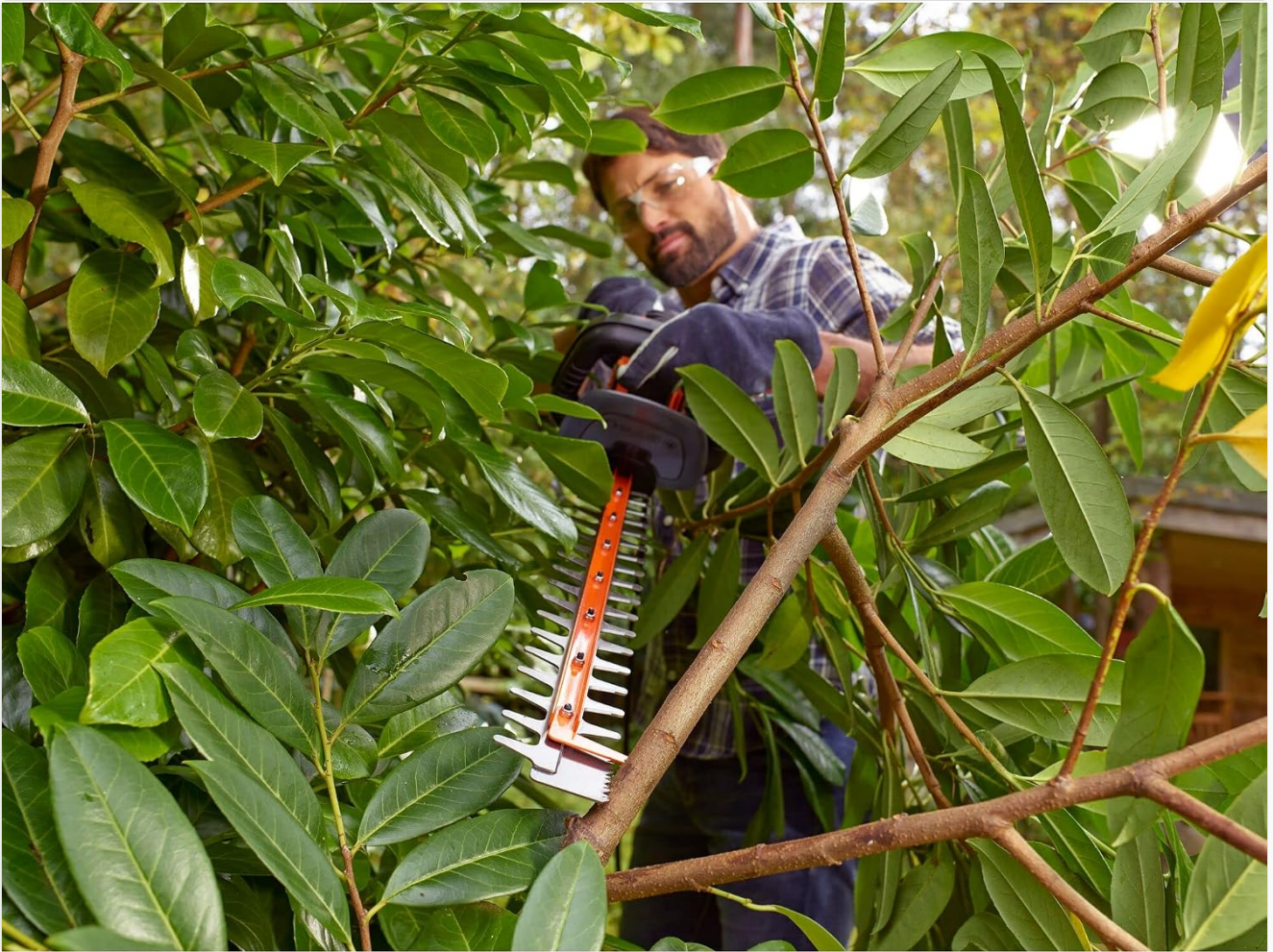
Image 4.5: A user utilizing the saw tip feature of the hedge trimmer. The image shows a person using the specialized tip of the blade to cut a thicker branch, demonstrating the tool's versatility.
