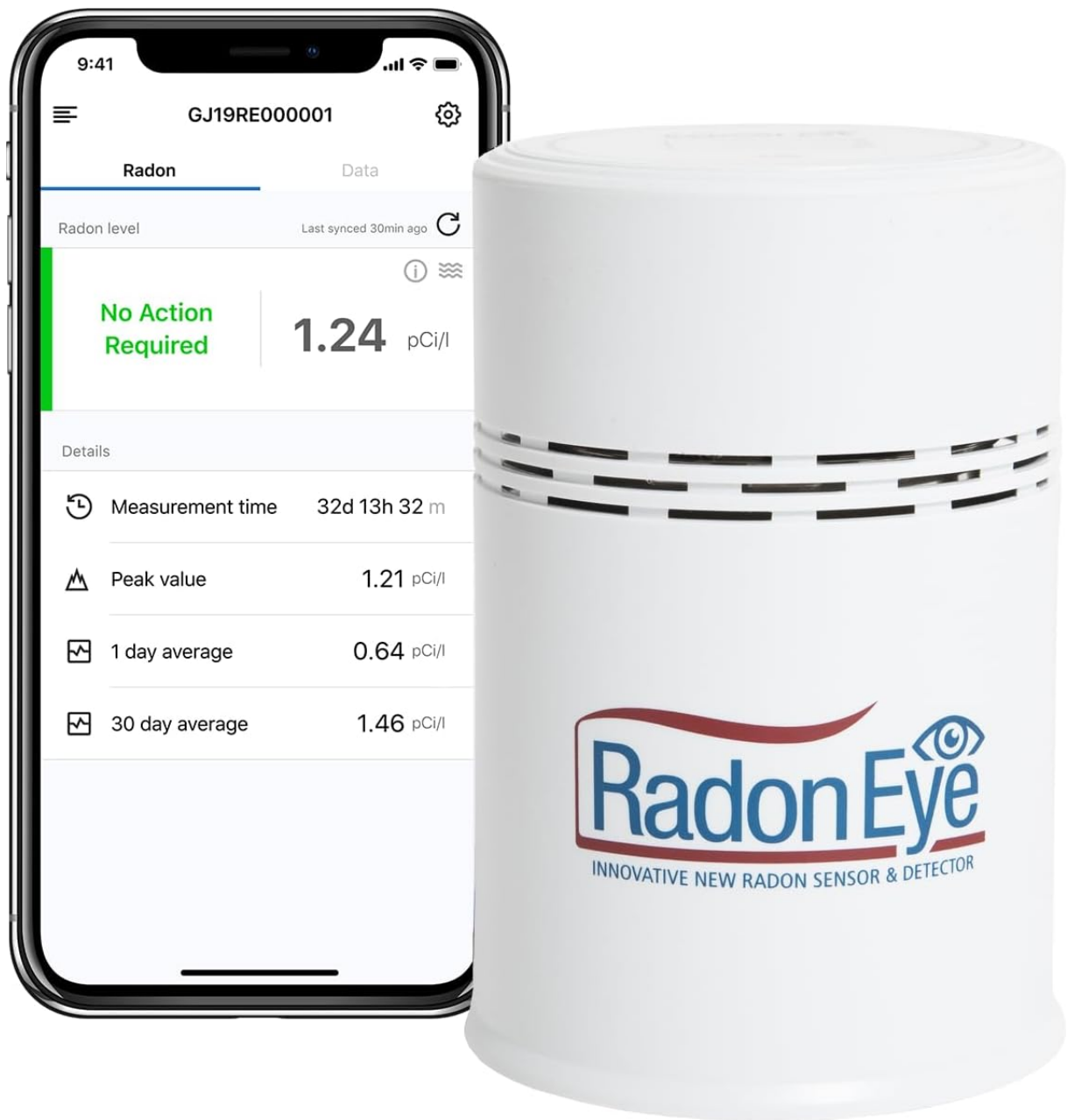
Image 5.1: The RD200 device alongside its mobile application, showing current radon levels and monitoring status.
