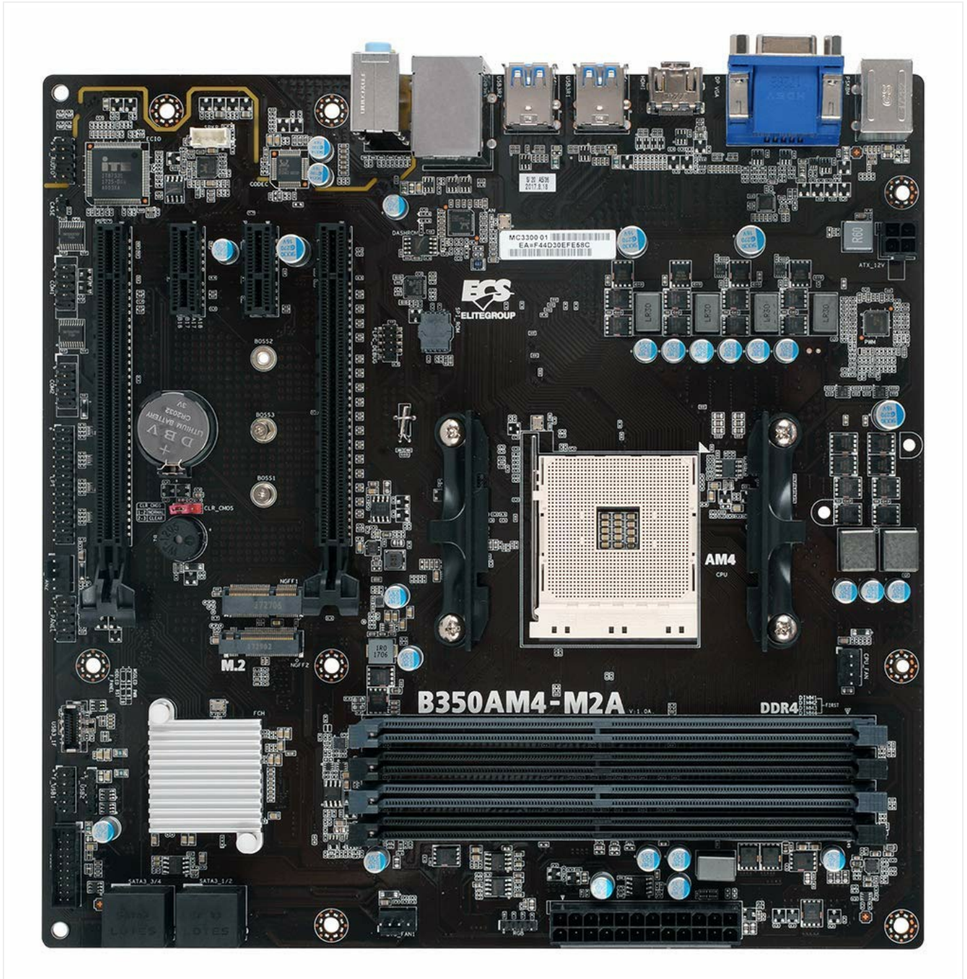
Figure 2: The AM4 CPU socket and surrounding area on the motherboard, where the processor is installed.
