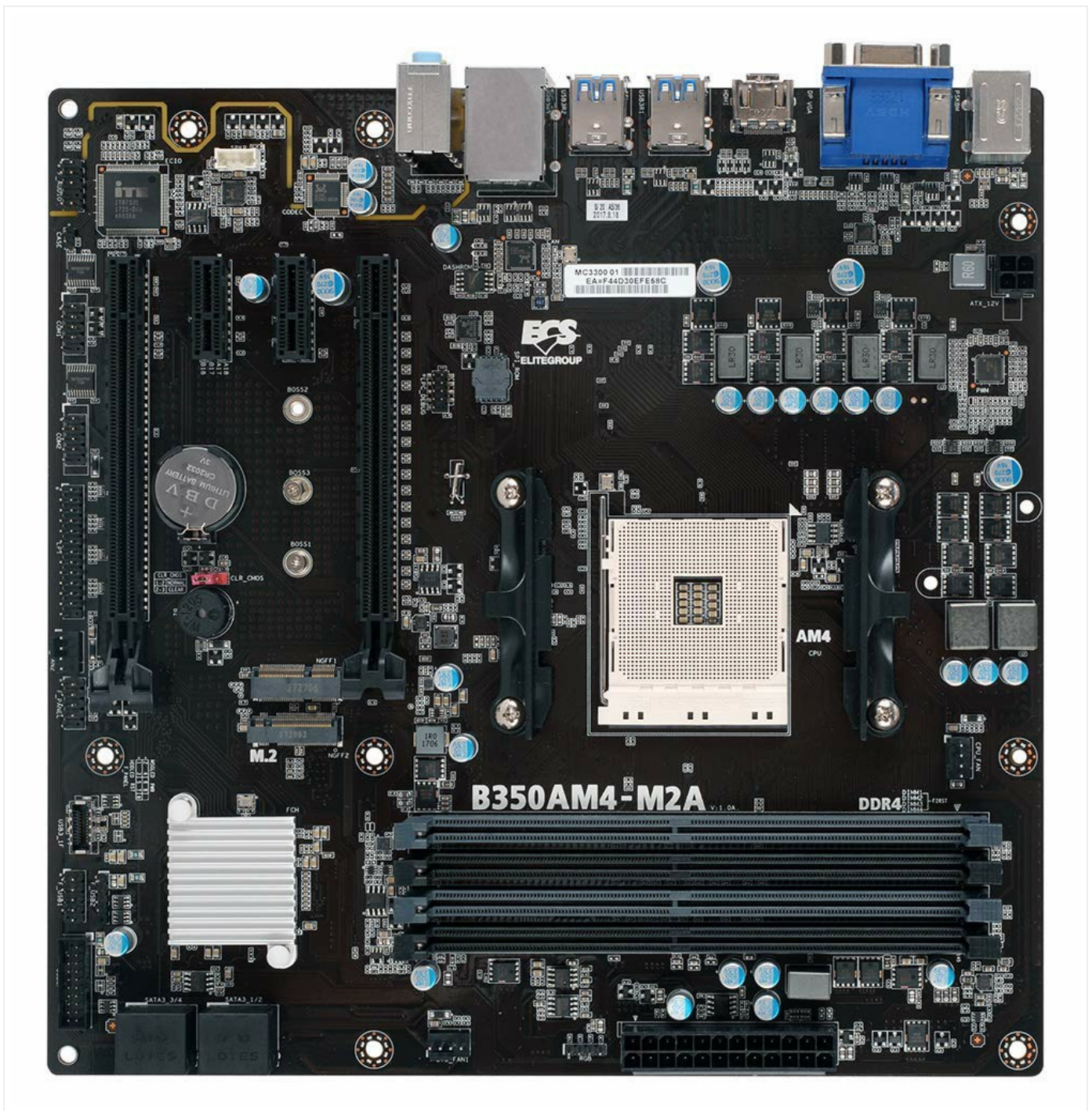
Figure 3: Location of the four DDR4 DIMM slots for memory installation.
