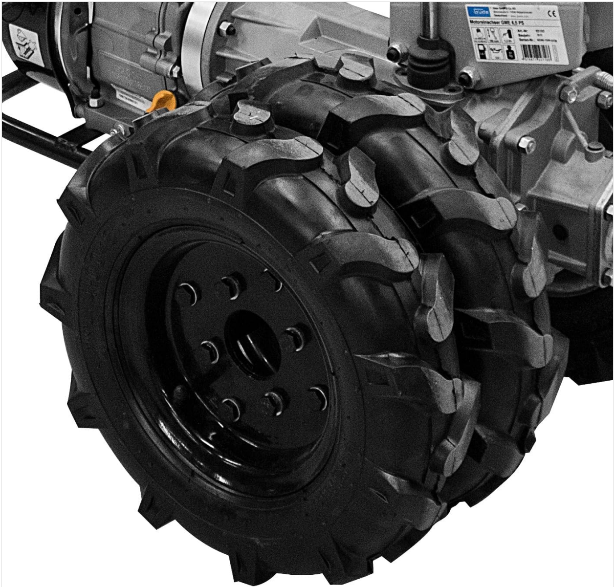
Figure 2: Close-up view of the double wheel assembly, illustrating how the additional wheel is mounted alongside the primary wheel.
