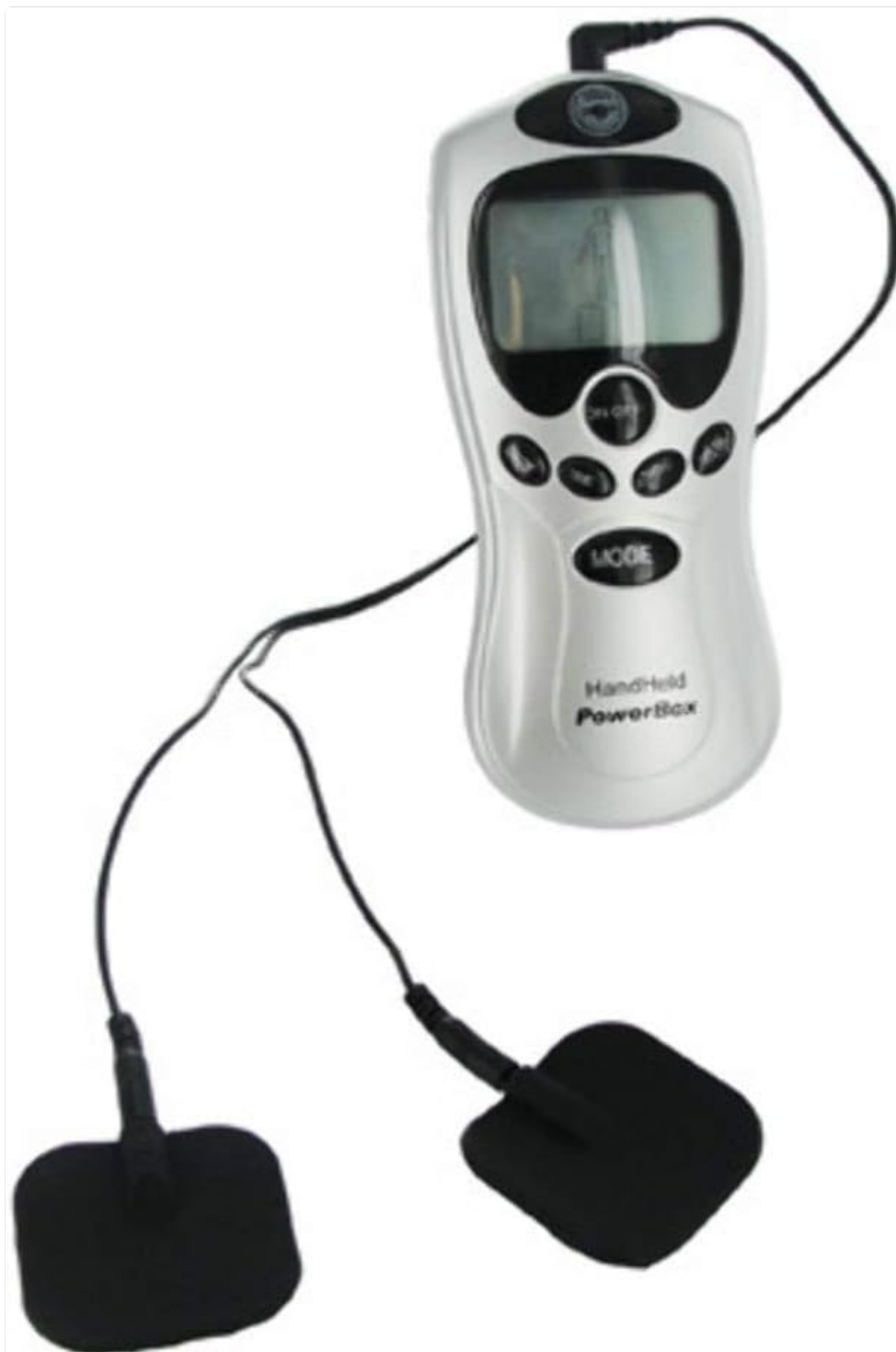
Figure 1: Front view of the E-STIM unit, highlighting the display screen and control buttons including ON/OFF, MODE,
