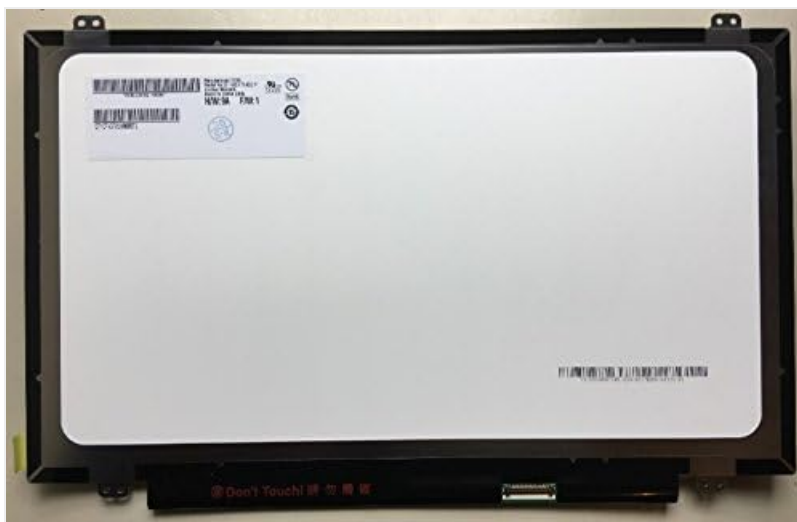
Image: The back of the LCD screen, displaying various labels and the location of the connector.
