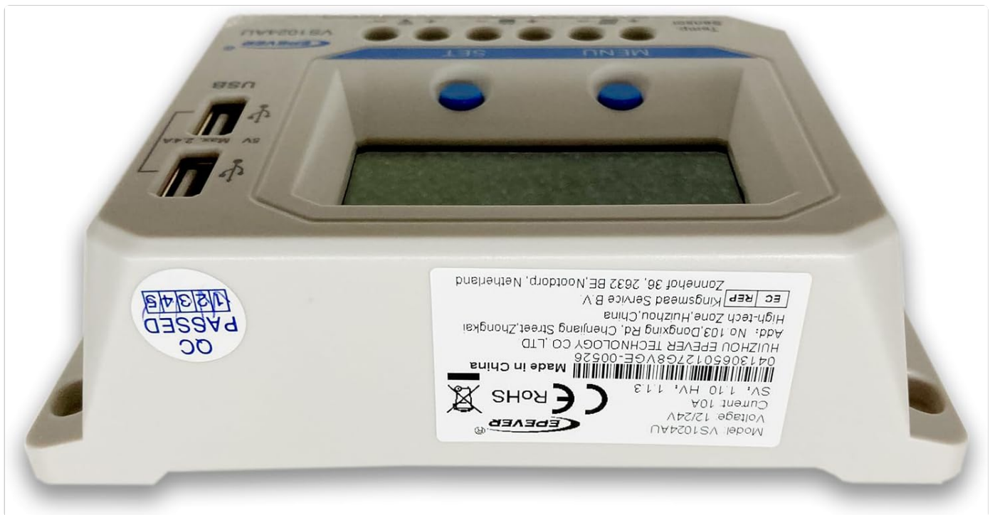
Figure 3.3: Side view of the controller, displaying the product label with model number VS1024AU, voltage, current, and various certifications including CE and RoHS. The label also includes a product identifier: 04130650127G8VGE-00526.
