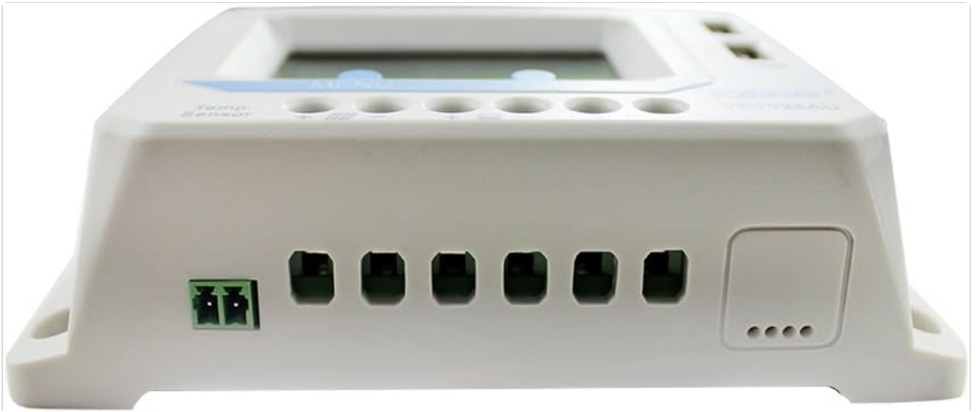
Figure 4.1: Bottom view of the EPEVER VS1024AU, illustrating the terminal connections for the temperature sensor, solar panel, battery, and DC load. Note the positive grounding configuration.
