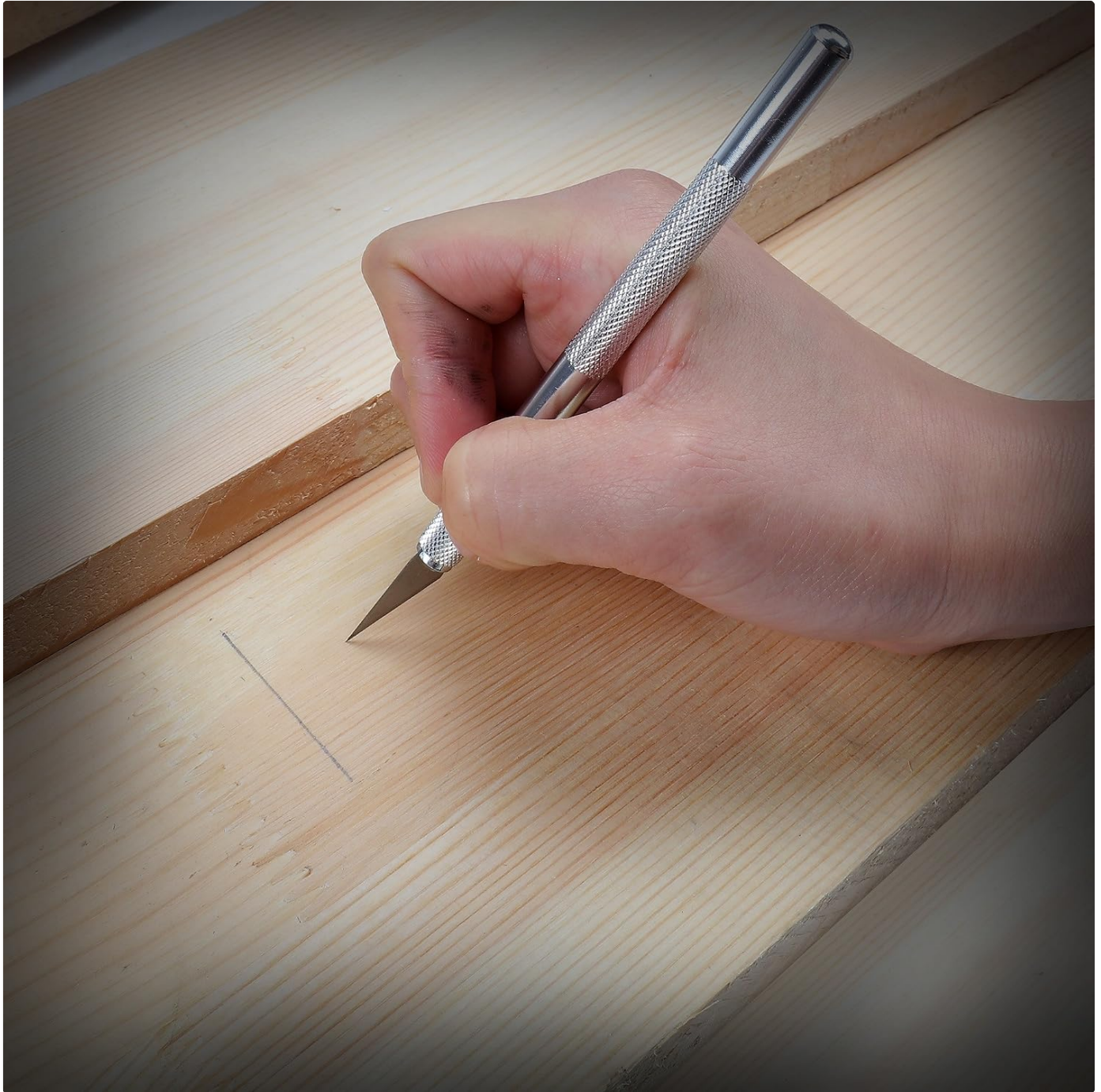
Figure 3: Using the precision knife for detailed work.
