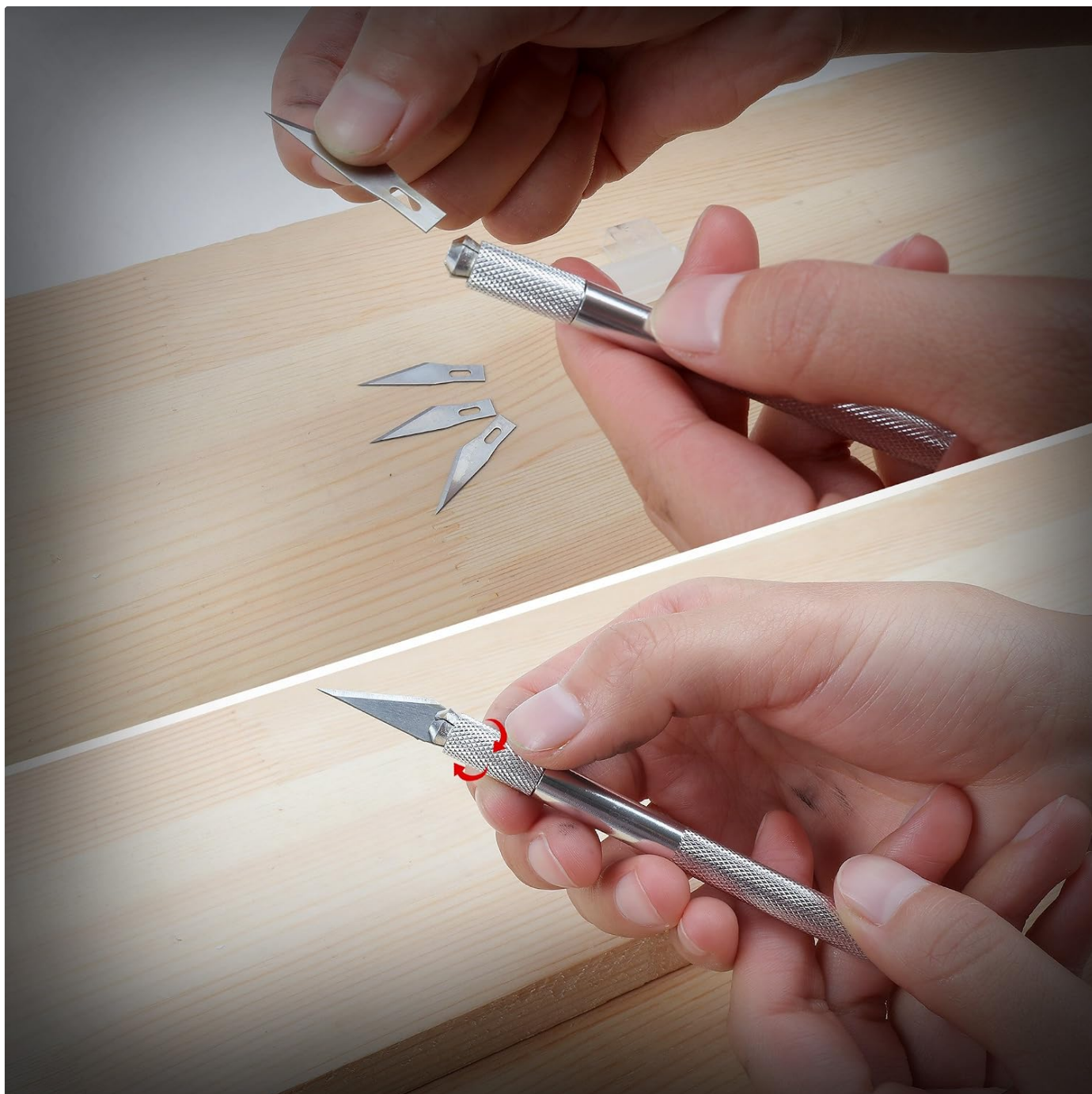
Figure 2: Installing a blade into the precision knife.
