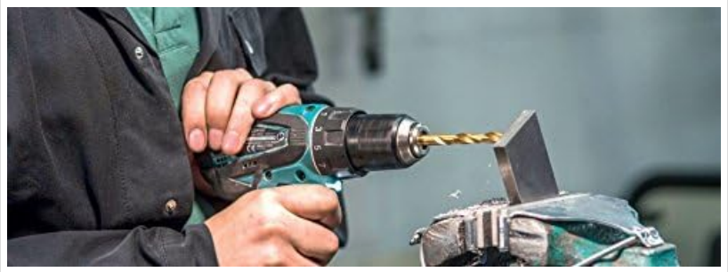
Image: A person using a cordless drill with a Heller drill bit to bore into a metal workpiece secured in a vise, demonstrating proper drilling technique.
