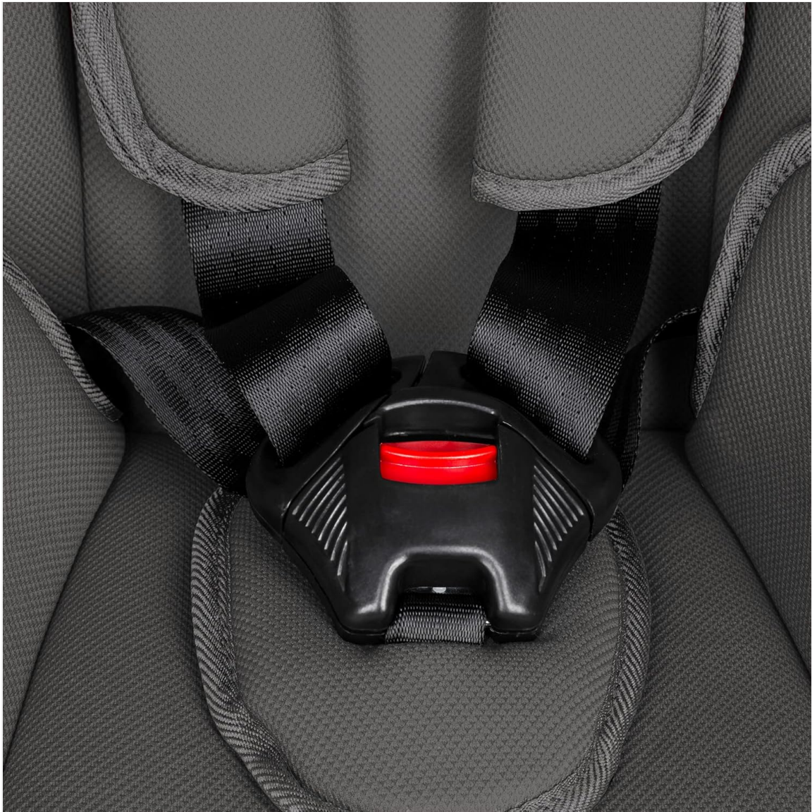
Figure 4.1: Detail of the 5-point harness buckle for Group 1 usage.
