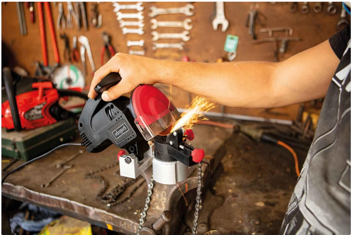
Image: The Scheppach KS1200 in action, demonstrating the precise grinding of a saw chain tooth. Sparks are visible, highlighting the importance of the spark screen and eye protection.
