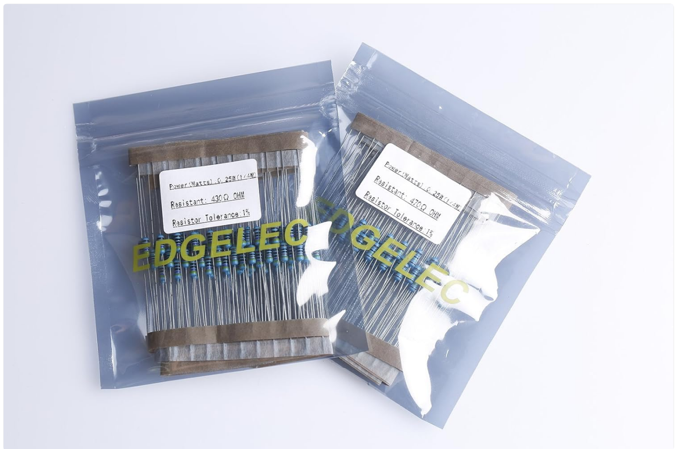
Figure 2.1: Included 430ohm resistors for current limiting.
