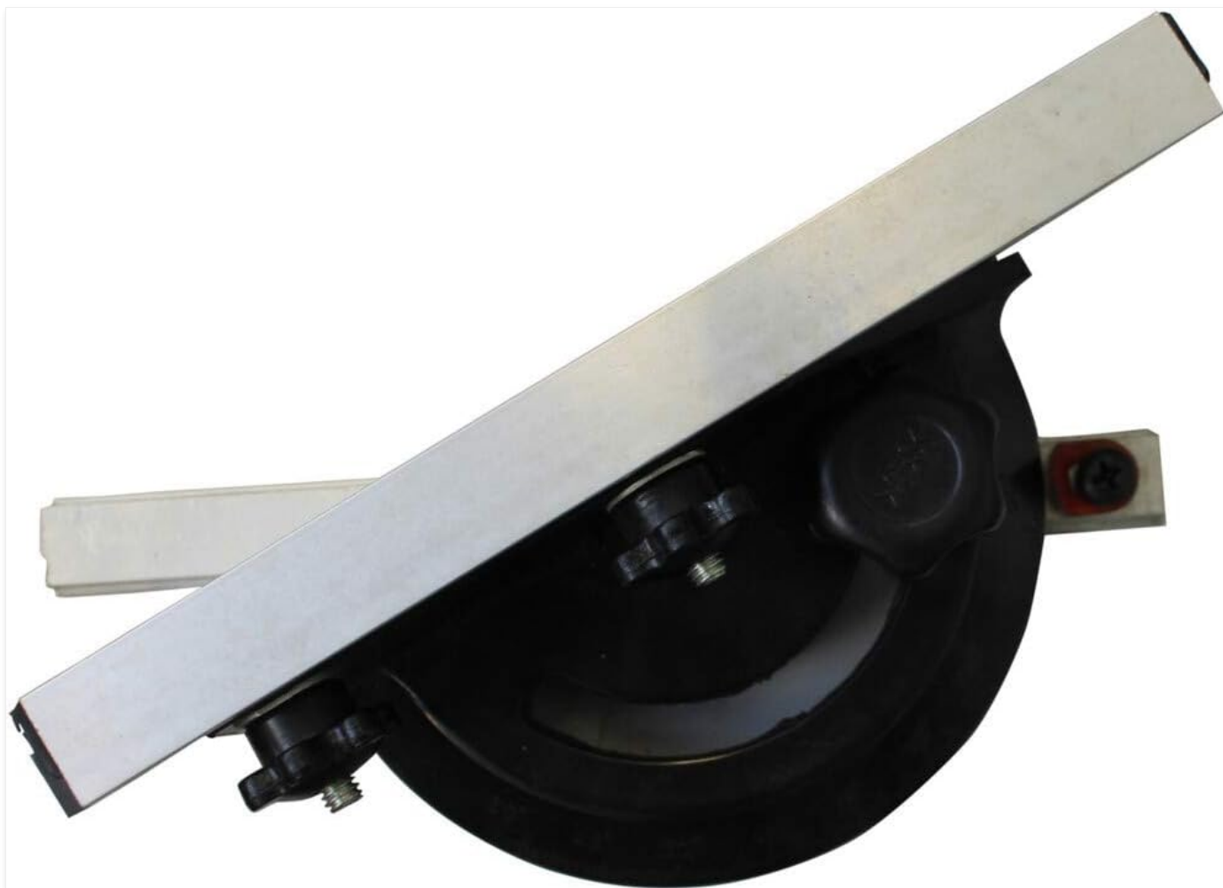
Figure 1: Scheppach 4901501701 Band Saw Cross-Cutting Gauge. This image displays the cross-cutting gauge, featuring a silver-colored metal fence attached to a black, semicircular base. The base includes two black adjustment knobs, allowing for precise angular settings. A metal bar extends from the base, designed to slide into the band saw's miter slot.
