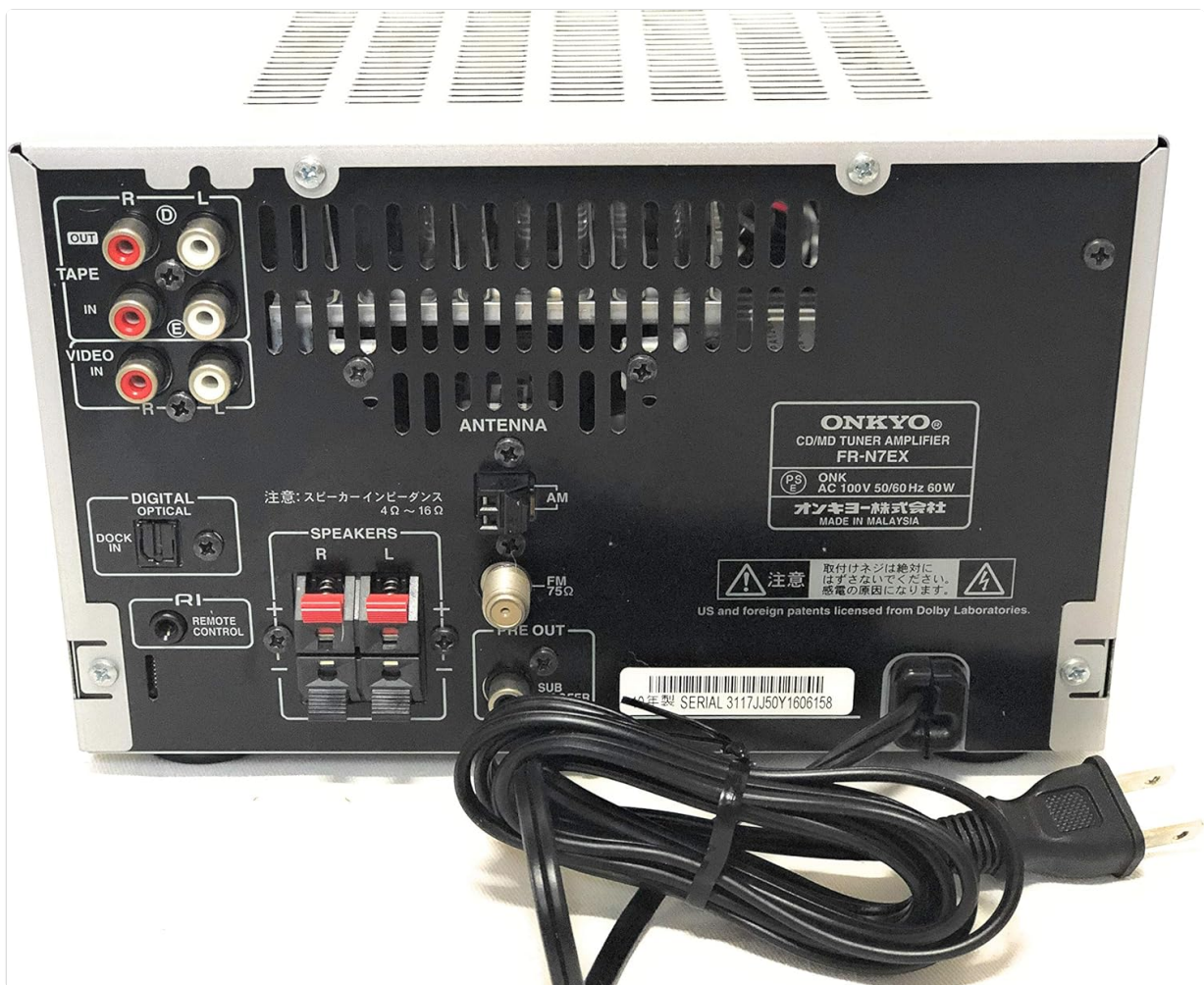
Figure 1: Rear panel connections, including speaker terminals (red and black clips) and various audio input/output ports.
