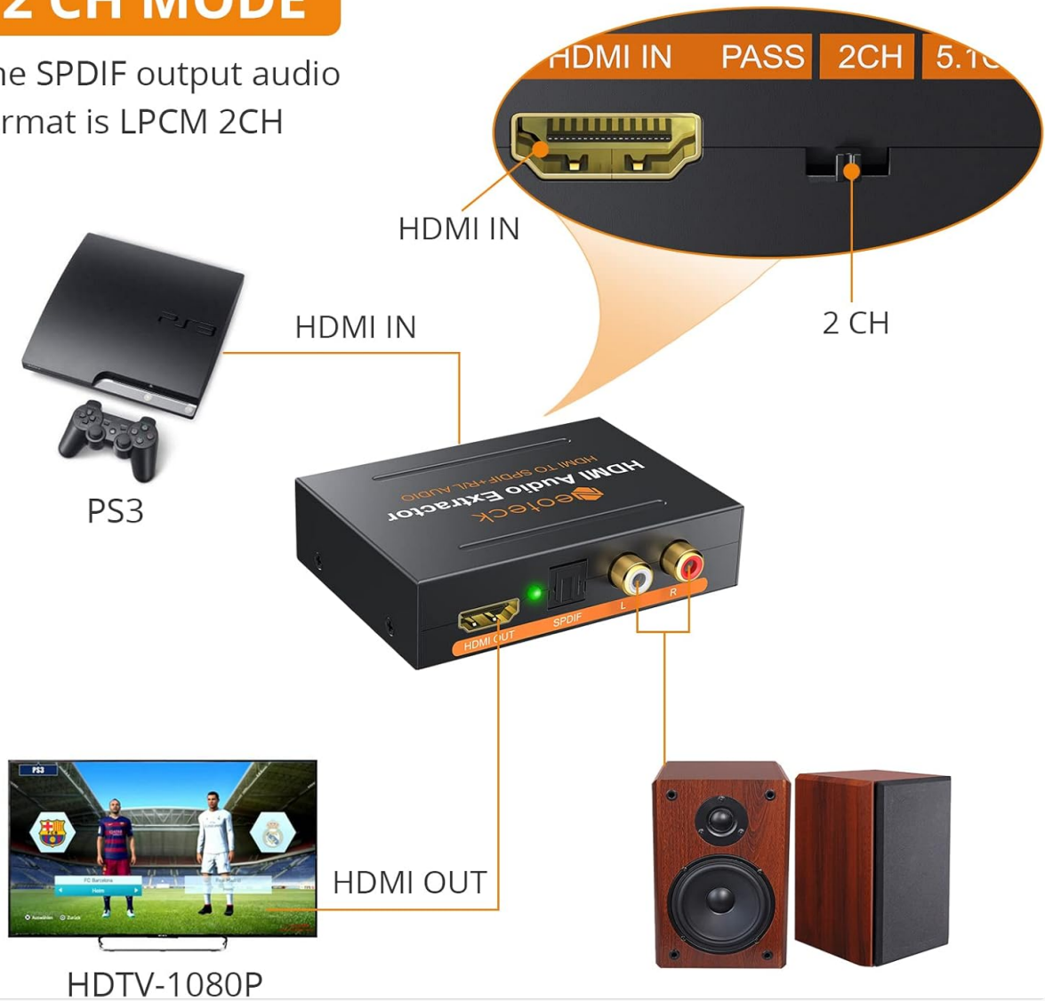
Figure 3: Connection diagram for 2CH mode. A PS3 connects to the HDMI IN. HDMI OUT connects to an HDTV. The L/R RCA outputs connect to stereo speakers. The EDID switch is set to 2CH.
