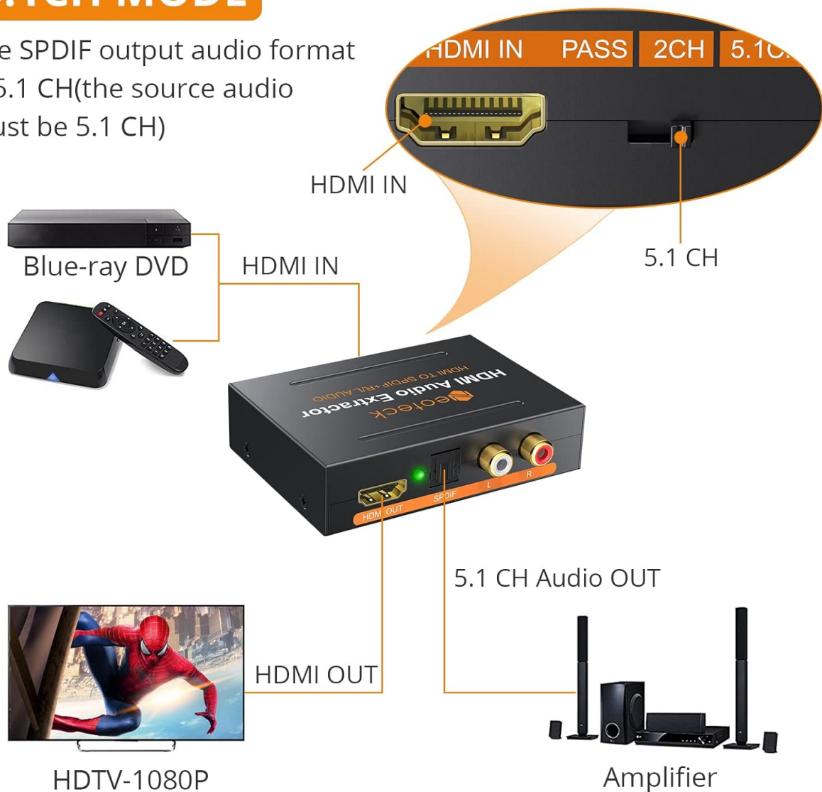
Figure 4: Connection diagram for 5.1CH mode. A Blu-ray DVD player connects to the HDMI IN. HDMI OUT connects to an HDTV. The SPDIF output connects to a 5.1 channel amplifier. The EDID switch is set to 5.1CH.
