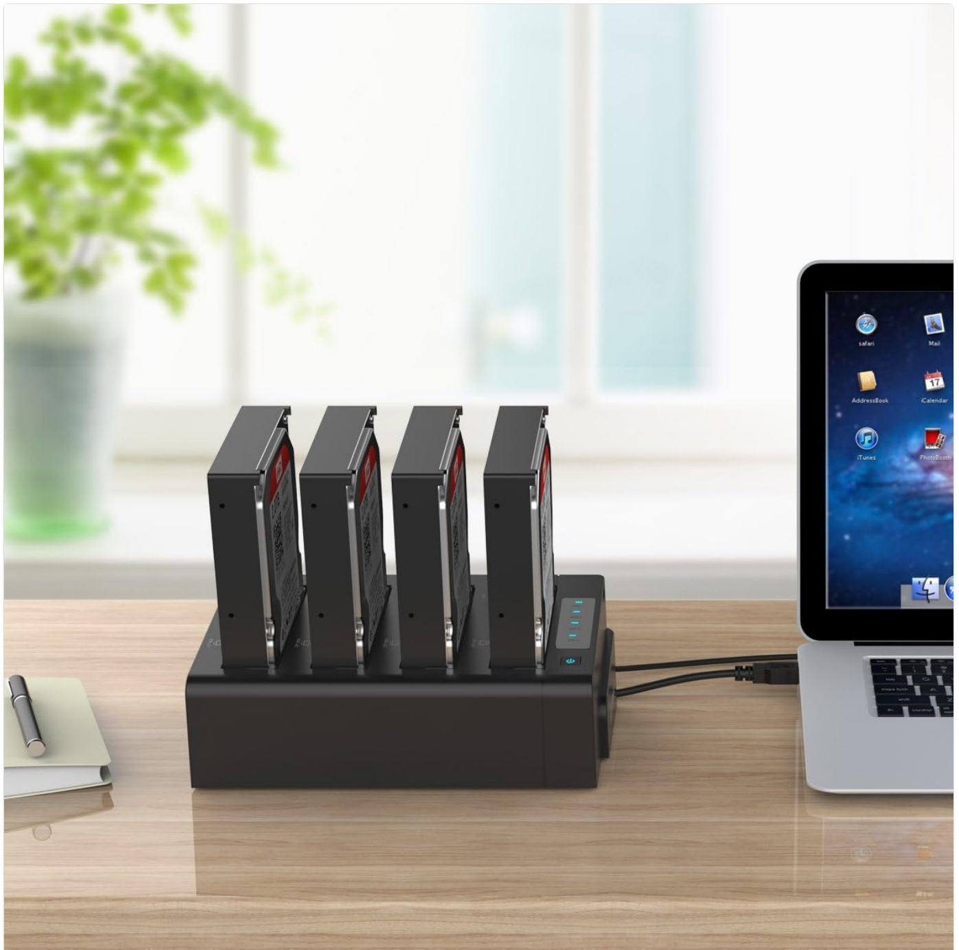
Figure 7: Docking Station in PC Mode
