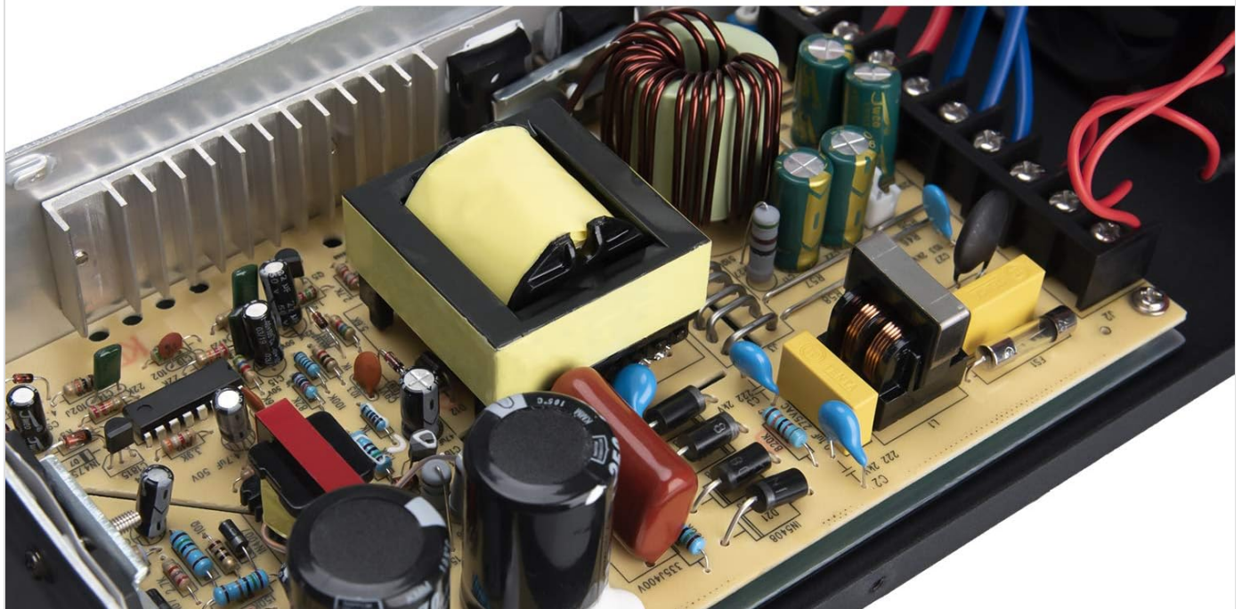
Figure 5.1.1: Diagram illustrating various protection mechanisms including temperature, reset, short circuit, input overvoltage, input anti-counter, input overcurrent, battery, and PTC protection. Below, an image of the internal circuit board shows components like capacitors, chips, and radiators designed for stable and safe power delivery.
