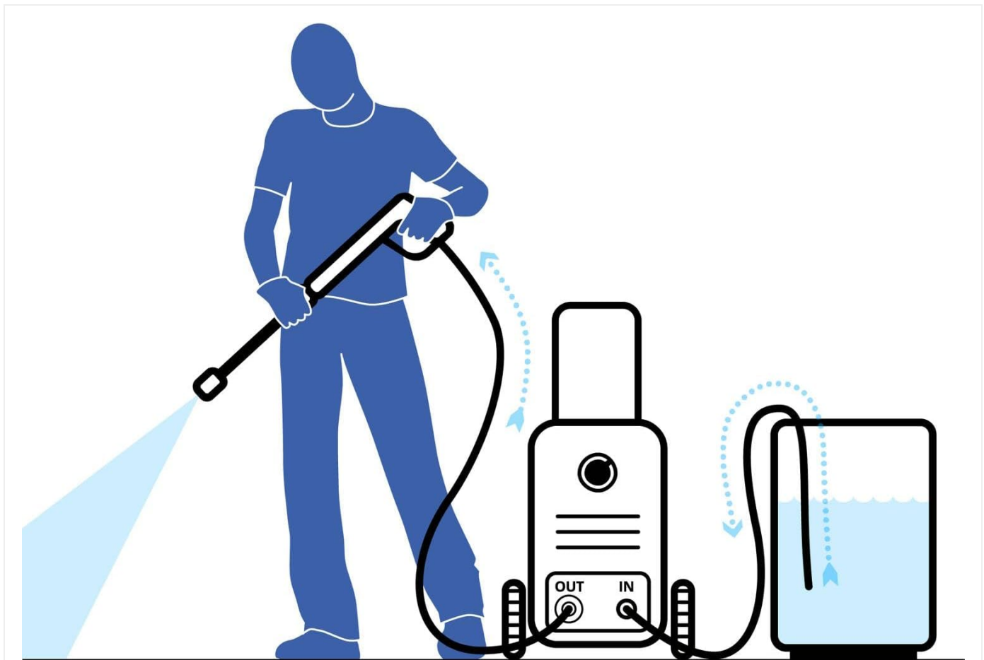
Figure 3.1: Diagram illustrating how to connect the pressure washer to a static water source, such as a water tank, for self-priming operation.
